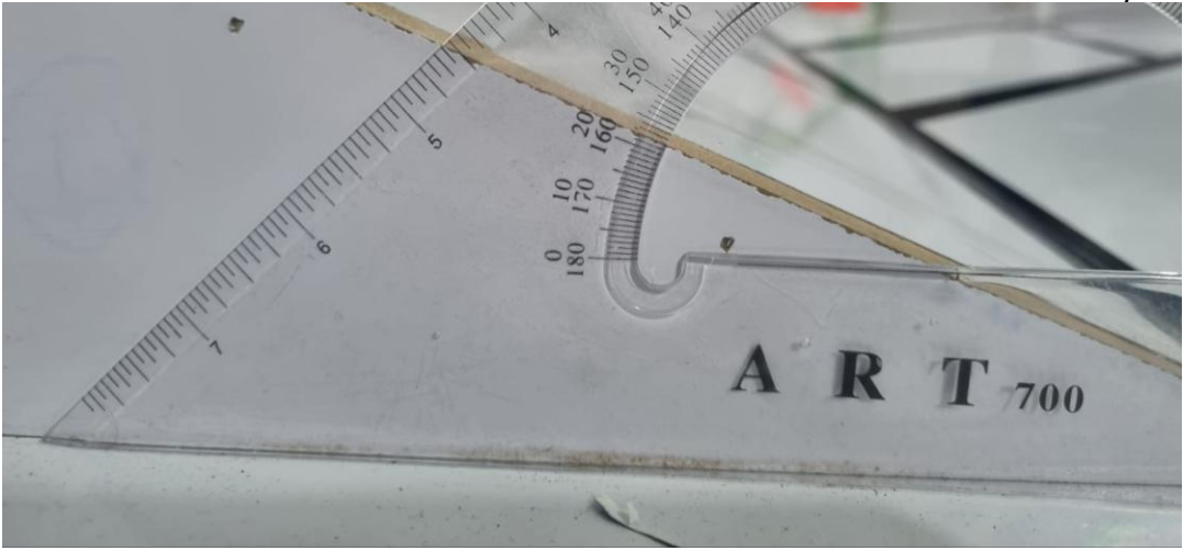
Figure 3: Ramp Angle (22 degrees)
